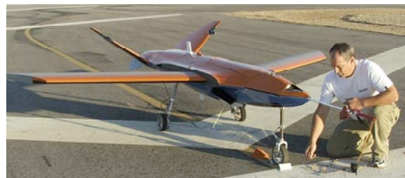
Figure 6 Morphing RPV Developed by NextGen Aeronautics in the DARPA MAS III Program
